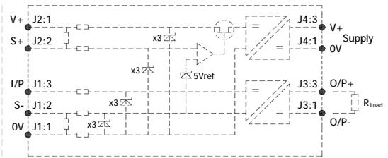
**Putting Into Service:** The sensor must be used with a galvanic isolation barrier designed to supply the sensor with a nominal 5V and to transmit the sensor output to a safe area. The barrier parameters must not exceed:-
