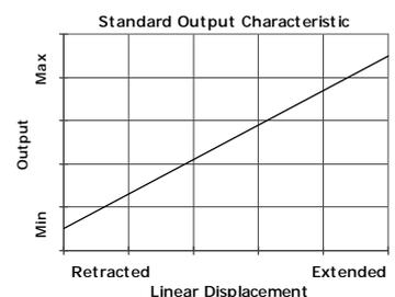
**Output Characteristic:** Target position at start of normal travel is 36.0 mm from seal face.
